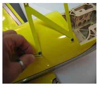
$\Box$  step 5 Locate and fix the two aluminium pieces (that after need to be glued into top wing), with 3mm screws, as per picture.
