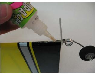
□ **step 7**Carefully locate the rudder and glue the hinges with some drops of thin CA.
