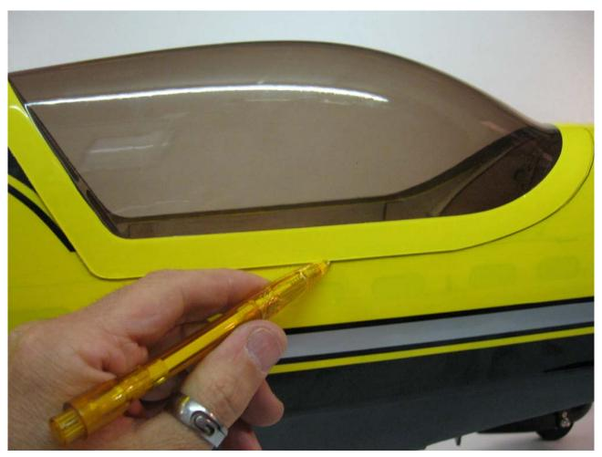
$\square$  step 3 Send the canopy on the inside and the oracover surface on fuselage.
