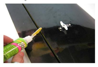
□□□□ **step 8**Install the control horn as per picture.
