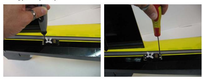
$\square$  step 3 Glue the fibreglass horn with medium CA into the elevator.
