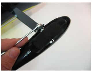
□□ **step 5**Hold the wheel pant parallel to the fuselage and drill the location for the wheel pant screw using a 1,5mm drill bit. Attach the wheel pant to the landing gear using a 2mm short self-tapping screw.
