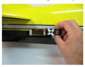
$\Box$  step 2 Drill the location for the four self-tapping screw using a 1.5mm drill bit and install the servo into the wing panel as per the picture.
