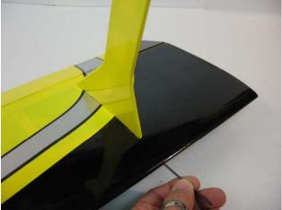
$\hfill \Box$  step 8 Install the top wing and test assembling and alignment.
