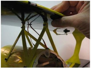
$\square$  step 9 Check incidence of wings with the provided plywood support, included in the hardware.
