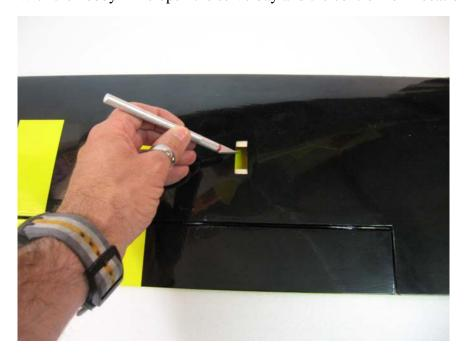
$\square$  step 3 With the hobby knife open the servo lead exits in the bottom & top wing.
