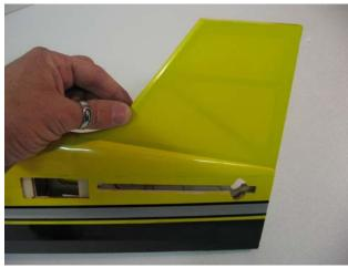
$\Box$  step 4 With the hobby knife cut a groove of 20mm length into the rudder. Drill in the rudder, 20mm from the bottom, the location for the tail wheel using a 2mm drill bit.
