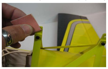
$\Box$  step 7 With the hobby knife cut holes the pylons location into top and bottom wing, and install the pylons in the bottom wing with the pins, as per picture.
