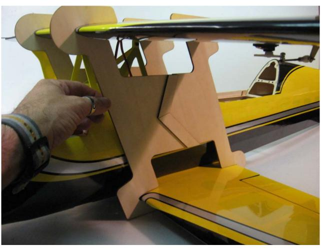
$\Box$  step 10 Once satisfied with the alignment and incidences, disassemble the top wing and put the 5 minutes epoxy glue in the two aluminium locations and reassemble it rapidly, repeating step 8 and step 9.
