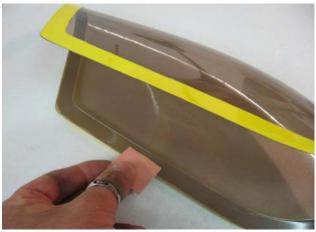
☐ **step 4**Using 5 minutes epoxy glue carefully the canopy on the fuselage.
