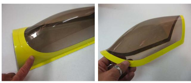
$\square$  step 2 Locate the canopy on the fuselage and sign the border, as follow.
