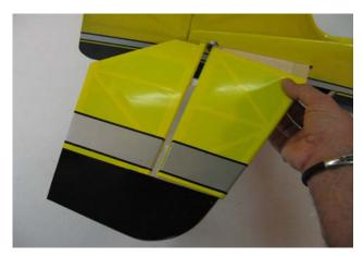
□ **step 4** Glue carefully the hinges in the stabiliser with some drops of thin CA.
