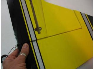
$\hfill\Box$  step 8 Drill the screw locations for the tail wheel using a 1,5mm drill bit, and install it as per picture.
