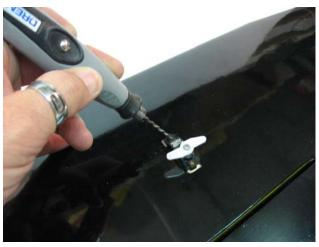
$\square\square\square$  step 7 Glue the fibreglass horn with medium CA into the aileron.
