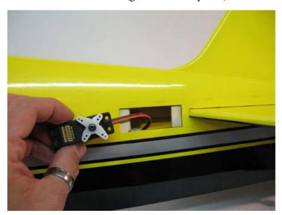
$\Box$  step 3 Drill the location for the four self-tapping screw using a 1.5mm drill bit and install the servo into the wing panel as per the picture.
